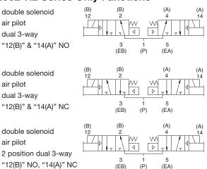
5 Ported, 2 and 3 position, 4-way and dual 3-way, Packed Spool Cv: 0.25 (4-way)
