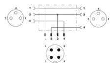
M12 to M12 Cable Splitter - Pin Out M12 to M8 Cable Splitter - Pin Out TA04XXMIEKC03000 (Male to Female View)
