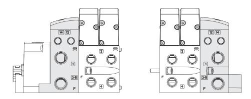
Shaded components are described by the manifold assembly number. The communications module is described by the Electronic Interface model number designation.
