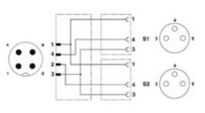
M12 Field Wireable (IDC) - Pin Out TA04F200000081E (SPEEDCON®) (Male View)
